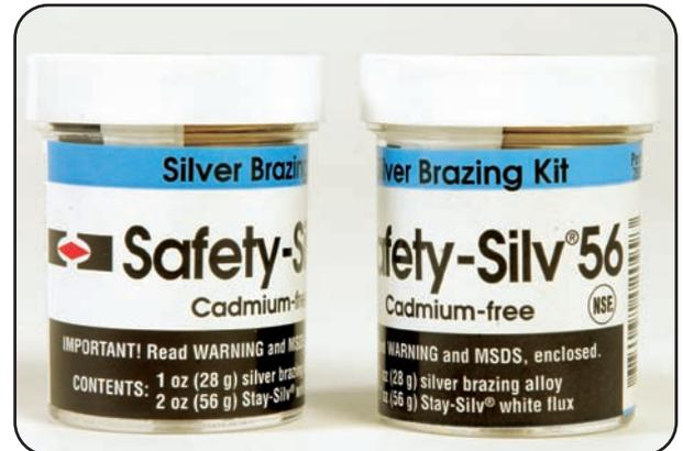
◆ **SAFETY-SILV® 56** - This high silver (56%) content alloy makes first quality brazes. It is free-flowing with unequalled capillary attraction and deep penetration. Ductility is high, corrosion resistance suitable for all but strong chemical applications. Offers highest elongation of silver brazing alloys. Suitable for use in the food processing industry. The silver color is an excellent match for stainless steel and silverware applications. NSF Certified to NSF C2.
